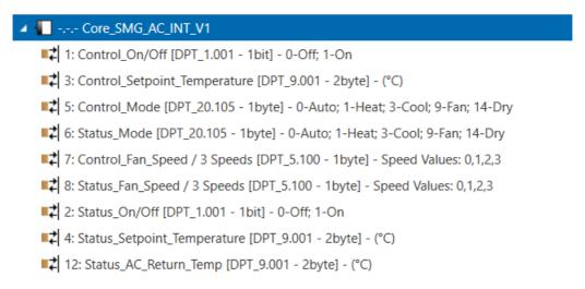
With the default group objects and specified data types, basic functions such as on/off, control modes, fan speed, target temperature and ambient temperature of the indoor unit can be controlled, and their instantaneous values can be read.
